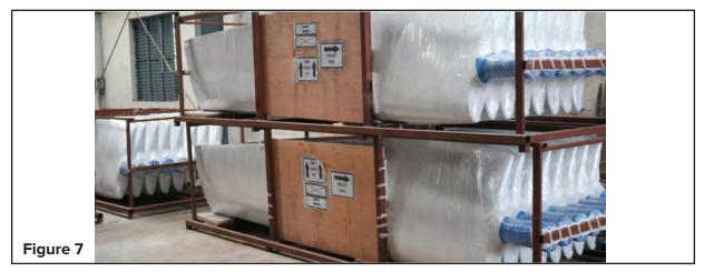
The fan blades can be lifted from the packing by placing a single sling around the blade. Position the sling as such that the blades tip is somewhat hanging down which makes it easier to move blades around.
