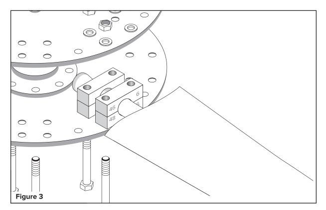
10 Measure the final fan diameter. minimum clearance between all blade tips and fan cylinder is recommended.
